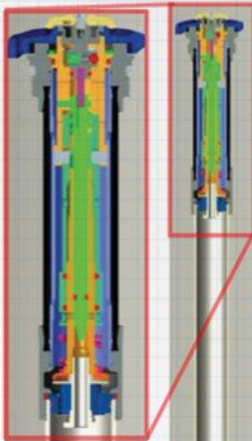
Vertical cut-away of Charger damper
